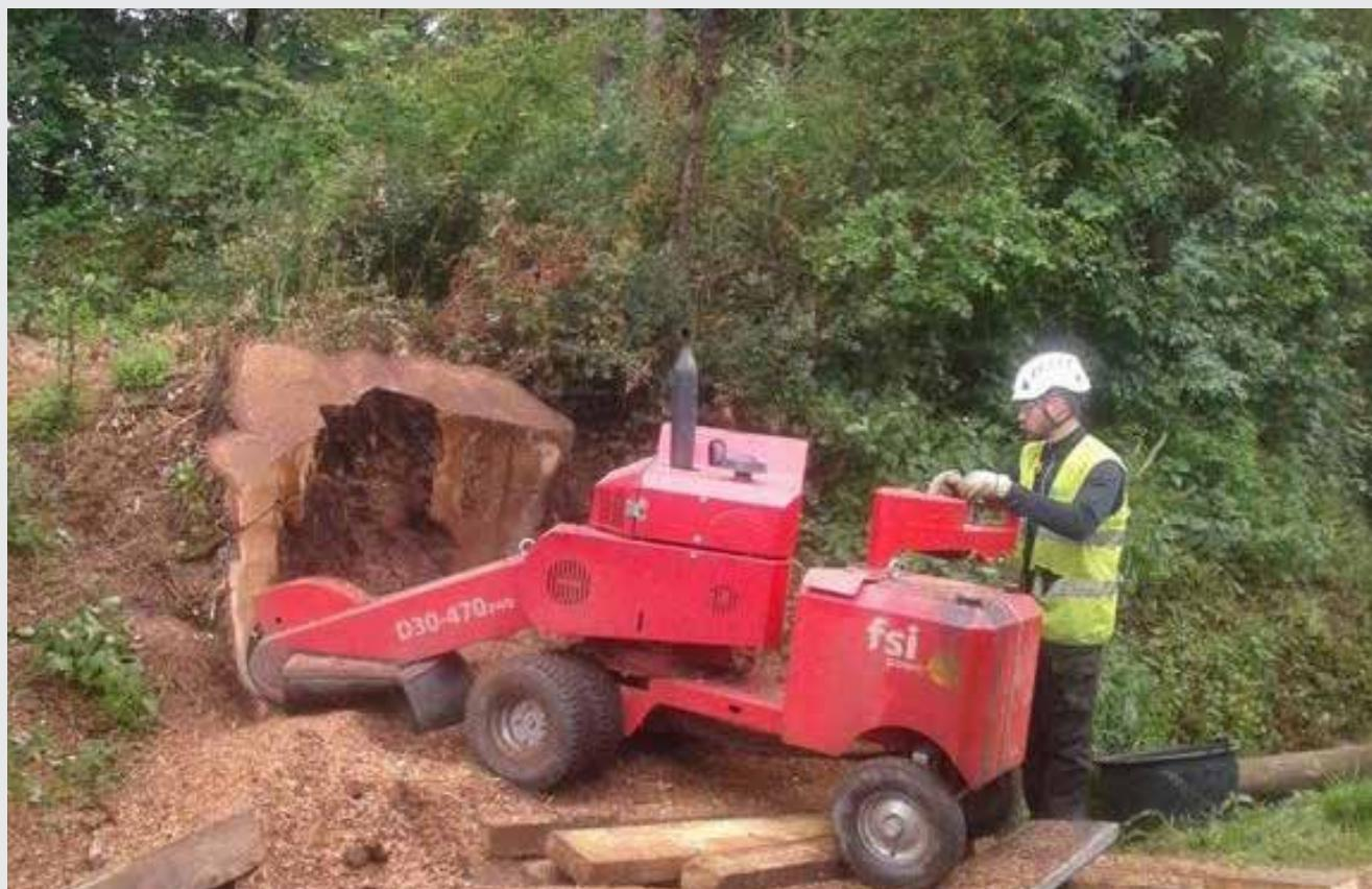
**LES MACHINES NE SONT PAS DES MONSTRES SURDIMENSIONNÉS : PAR EXEMPLE, LA POSSÉDÉTÉ DE SOULEVER LA ROGNEUSE DE SOUCHES PAR-DESSUS UN MUR, DE RETIRER LES ROUES JUMELÉES, DE MANŒUVRER FACILEMENT AUTOUR DES SOUCHES ET DE TRANSPORTER L'APPAREIL SANS DIFFICULTÉ EN FONT UN OUTIL INDISPENSABLE SUR TOUT CHANTIER.**
